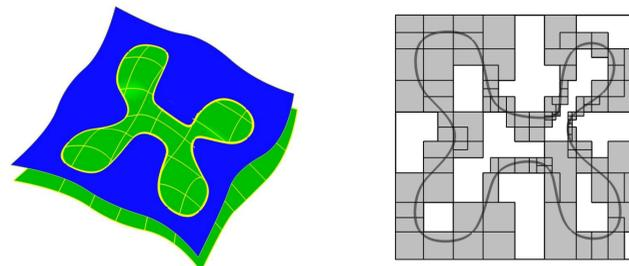
Two B-splines surfaces with closed curve intersection (left). Preimage in the parameter space of the **blue** surface.
